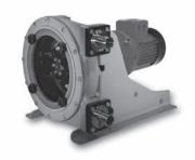
The DULCOFLEX DFC is a hose pump designed for difficult pumping applications. It incorporates a roller design which eliminates the need for cumbersome lubricants, unlike typical shoe pumps. The DFC can reach pressures up to 116 psi and flow rates up to 106 gpm and is ideal for difficult industrial and municipal applications.
