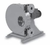
The DULCOFLEX DFD is a hose pump designed for pressures up to 232 psi and flow rates up to 160 gpm. The unique shoe design is made of steel for smoother and cooler compression. The DFD uses safe DulcoLube oil for the shoe lubrication. With suction lifts up to 29 feet, the DULCOFLEX DFD is a great choice for difficult pumping applications.
