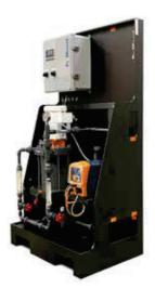
The ProMinent® ProMix™ is a pre-engineered polymer mixing system made for the water and wastewater markets. Designed as an in-line unit, the ProMix™ can be customized to meet most liquid polymer applications utilizing tubing or diaphragm pump technologies depending on the application requirement or customer preference. The unique mixing chamber allows for complete makedown of the neat or diluted polymer to guarantee a problem-free injection.
