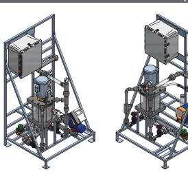
The ProMinent® ProMix™ is a pre-engineered polymer mixing system with intuitive controls. Designed as an in-line or makedown unit, the ProMix™ is engineered to meet liquid polymer applications utilizing diaphragm or progressive cavity pump technologies. The unique mixing regime delivers a highly activated polymer solution to every application with optimum performance
