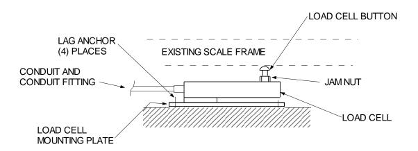
Step 4: Run conduit either to a junction box, or directly to the digital controller. This will be determined by individual installation conditions.
