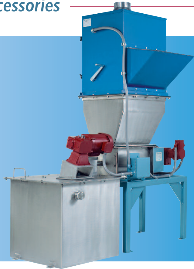
A Model W-105Z Feeder with a Dust Collector Bag Loading Station. The feeder meters product into a 100 gallon Dissolving Tank.
