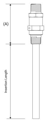
The IQ series non-retractable is well suited to small scale applications or those where the main can easily be depressurized to allow for servicing. The integrated check valve provides convenient isolation from the process pressure. Its size and availability in PVDF, C276, and Alloy20 make it ideal for sulfuric acid applications.
