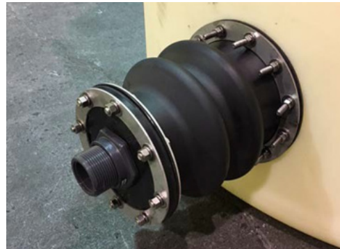
RE-INSTALL GASKET ON BHF THEN INSTALL; 6" GASKET, BLACK PE PLATE, AND 6" SPLIT RING'S USING THE PROVIDED HARDWARE. TIGHTEN NUT ONTO BHF. CONNECT PLUMBING TO FEMALE THREADED BULKHEAD FITTING. HYDRO TEST TANK
